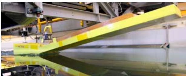
Figure 4. Wavedozer model attached to the towing tank carriage
