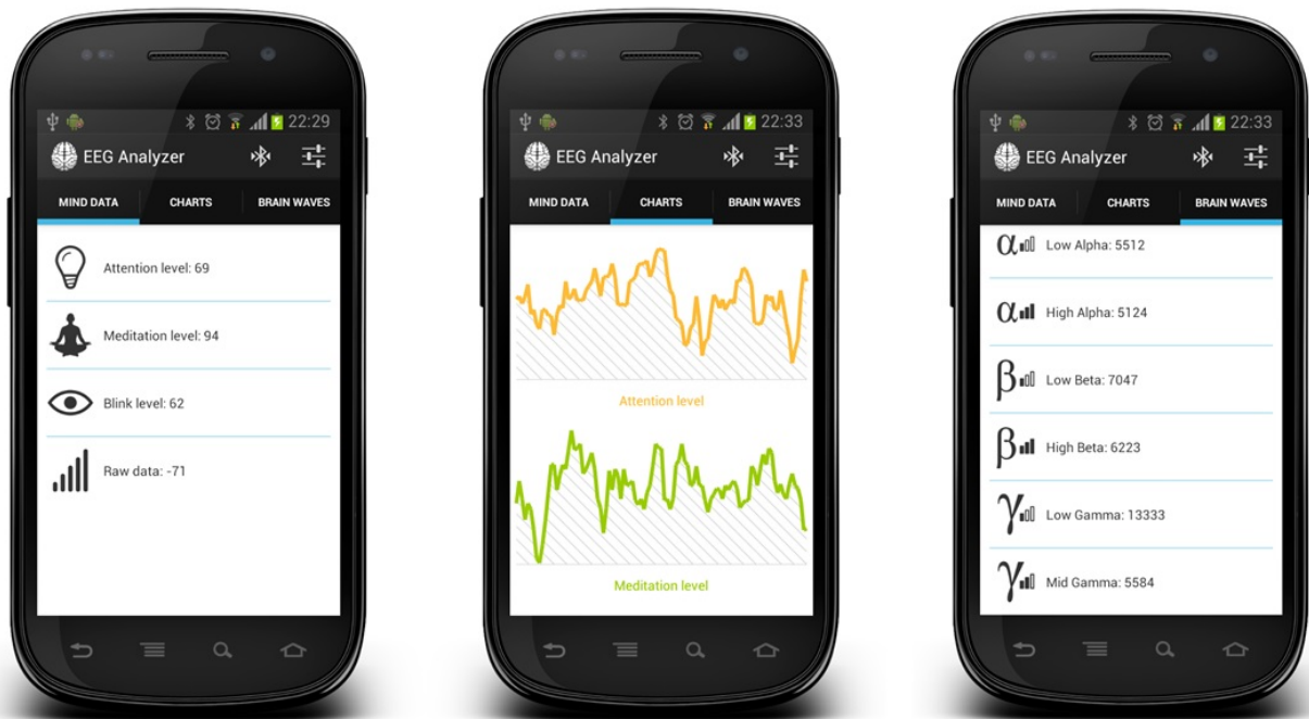
Fig. 2. Values of brain waves retrieved from MindWave Mobile device.
