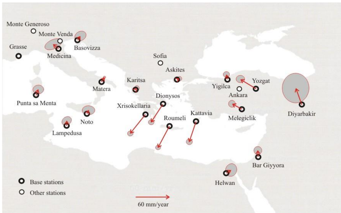
Fig. 3.2.3. SLR- and GPS-determined horizontal rates at WEGENER-MEDLAS stations. Horizontal motion vectors and error ellipses of Mediterranean stations relative to stable Eurasia.
