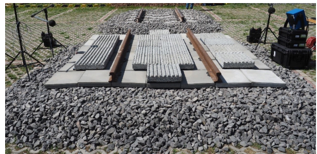
Fig. 7. View of the test stand with visible loudspeaker and microphones.
