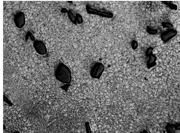
Fig. 7. Central zone of the AZ61 alloyed with SiC particles, scan rate: 0.75 m/min, laser power: 2.0 kW, mag. 500x
