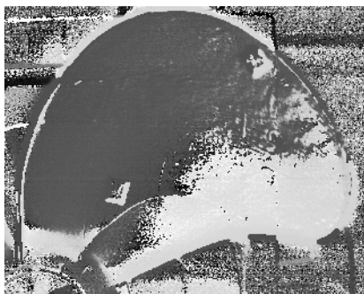
Fig. 5. Phase image showing time delays due to heat propagation
