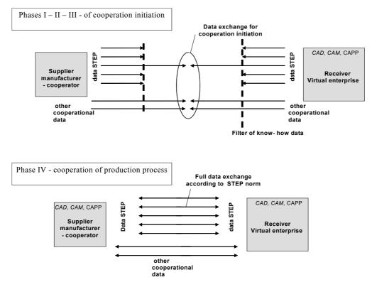
Fig. 7. Flow and standard of data in initiating and carrying out cooperation
