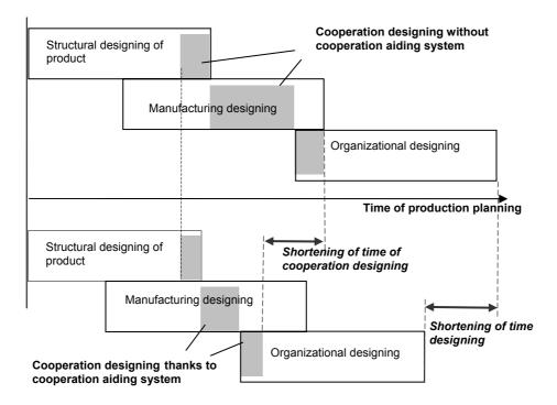
Fig. 9. Application of cooperation aiding system to shorten the time of production designing
