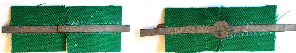
Fig. 6. Example views of a part of the connector prototypes (substrate and electro-conductive paths only)
