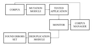
Fig. 4. Diagram of fuzzer generating test cases with an evolutionary algorithm
