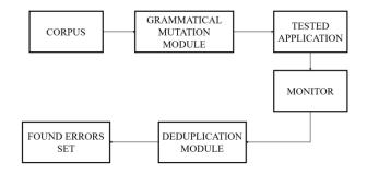
Fig. 3. Diagram of fuzzer generating test cases by grammatical method
