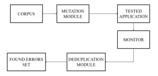
Fig. 2. Diagram of fuzzer generating test cases by mutation method
