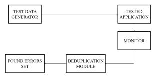
Fig. 1. Diagram of fuzzer based on a pseudo-random generator
