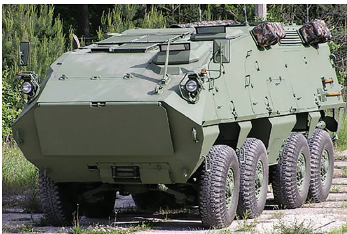
Fig. 2. Ryś armored personnel carrier in the base high version Source: Photo by WZM S.A.
