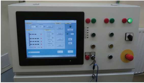
Fig. 7. The view of the operator panel (a) and the stand construction (b) for measuring burning rate for solid rocket propellants
