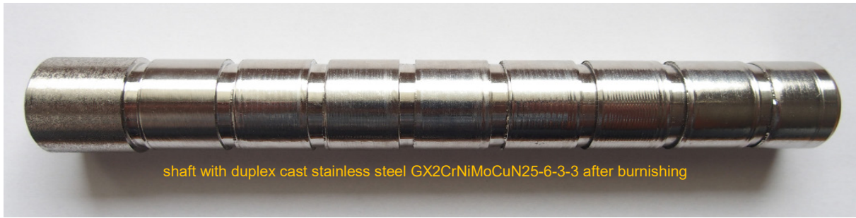
Fig. 2. The view of the sample duplex cast stainless steel series GX2CrNiMoCuN25-6-3-3 after burnishing process
