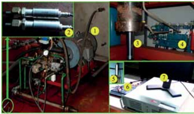
Fig. 3. Components of the actual steering system and experiment plant: 1. pump control subsystem; 2. hydraulic pressure sensor; 3. cylinder; 4. loading plant; 5. displacement sensor of cylinder rod; 6. data collector; 7. industrial computer
