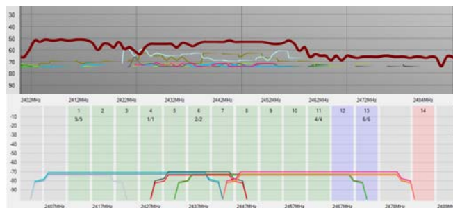
Figure 8. Measurements in moderate precipitation phenomena showed a power loss of about 10 to 12 dBm at 2,4 GHz
