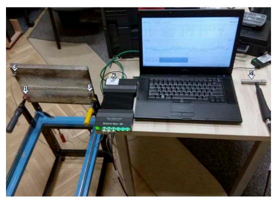
Figure 1. Stand for testing welded joints using vibration methods. The stand includes: 1– rack, in which plates (welding samples) could be mounted horizontally – four-point mounting or vertical – two-point mounting, 2 – Bruel & Kjear type 3050-A-vibration analyzer 60, 3 – accelerometers 4514-B, 4 – modal hammer (8206-002) with three exchangeable tips, i.e. metal, silicon and Teflon
