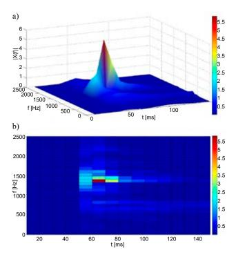
Figure 5. Time-frequency dynamic characteristics (a) 3D and (b) 2D for a welded plate with a non-defective welded joint (2202) for an impact made by an modal hammer with a metal head
