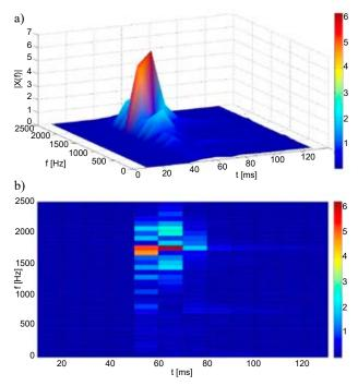
Figure 6. Time-frequency dynamic characteristics (a) 3D and (b) 2D for a welded plate with a fault (lack of side fusion [2127]) for an impact made by an modal hammer with a metal tip
