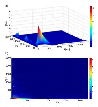
Figure 4. Time-frequency dynamic characteristics (a) 3D and (b) 2D for a plate with no welded joints (0) for an impact made by a modal hammer with a metal head
