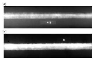
Figure 2. Radiographic photography of the welded joints for a) welded joint without faults (2202) and b) welded joint with incompatibility in the form of boundary bonding (2127)
