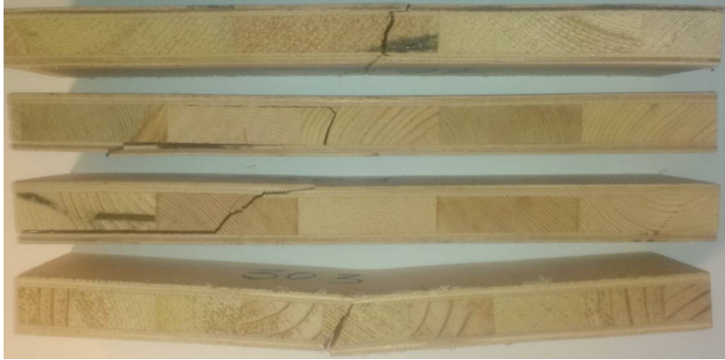
Fig. 11. The nature of the destruction of the specimens of the PCW-BB during the bending strength test
