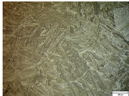
Fig. 5. Microstructure of steel with 5.01 Ni eqv. after quenching and tempering, quenching in quiet air
