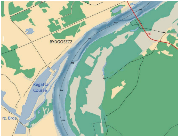
Fig. 7. Bathymetric plan of the pseudo-meander channel of the Vistula (Wisła) at the Gorge at Fordon on 770–773 km, regulated in the 19th century
