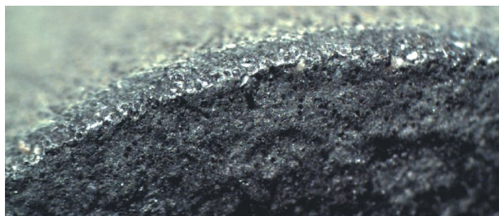
Fig. 4. Worn out edge of cutter after tests on Vosges sandstone
