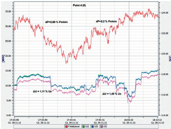
Fig. 2. Example waveform of active power and voltage changes in farm's PCC point at active power reduction to 50%
