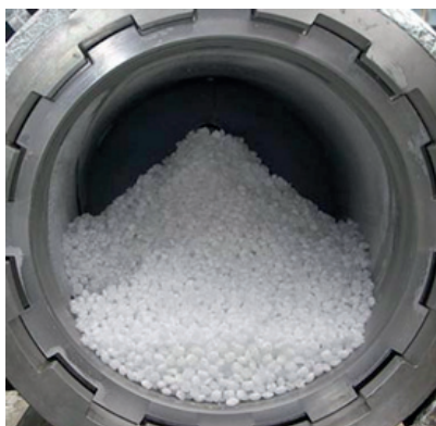
Fig. 1. The form of hydrate capsules within the container
