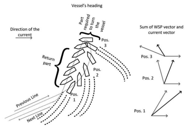
Figure 5. Tow movement and heading of a seismic vessel while conducting a "saving turn"
