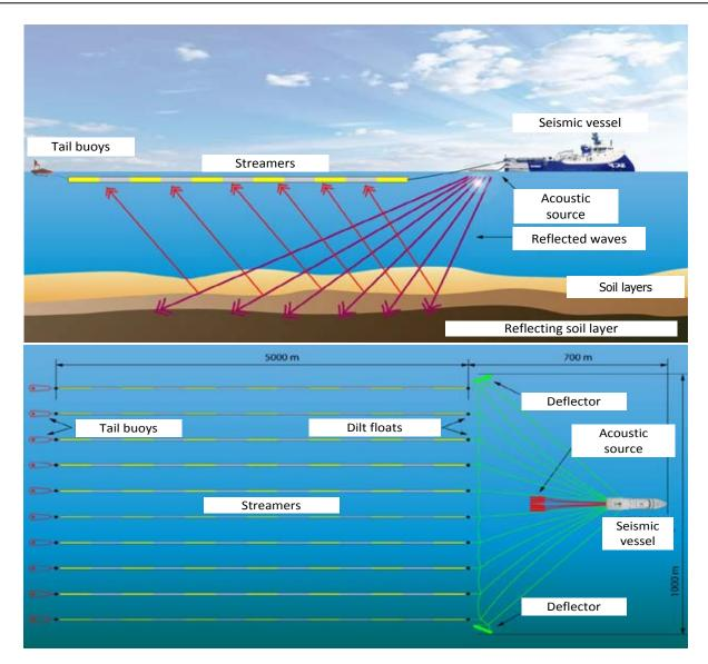
Figure 1. Example of a towed seismic spread and explanation of specific names
