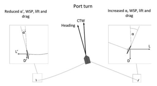
Figure 4. The hydrodynamic forces and angle of attack on deflector vanes during a port turn
