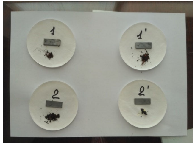
Fig. 2. Photos of specimens from pipe steels and corrosion products after testing
