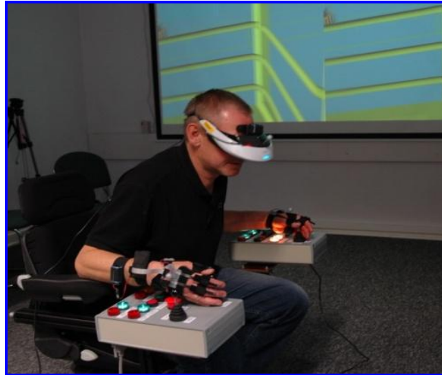
Fig. 6. A participant of the tests conducting an interactive simulation of using the virtual overhead crane
