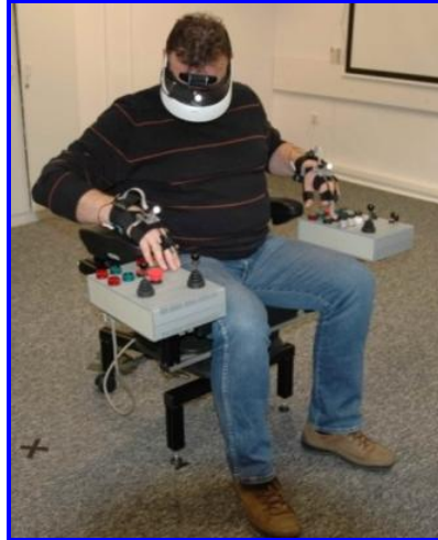
Fig. 2. View of the simulator's seat after the user sits and wears VR hardware
