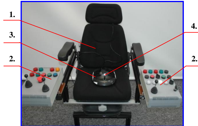
Fig. 1. View of the overhead crane simulator: 1 – seat of the simulator, 2 – real panels to control the virtual overhead crane functioning in the simulator, 3 – infohelmet, 4 – motion sensor of the tracking system
