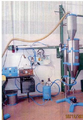
Figure 3. PEEN-IMP device for pneumatic peening (patent PL204718).
