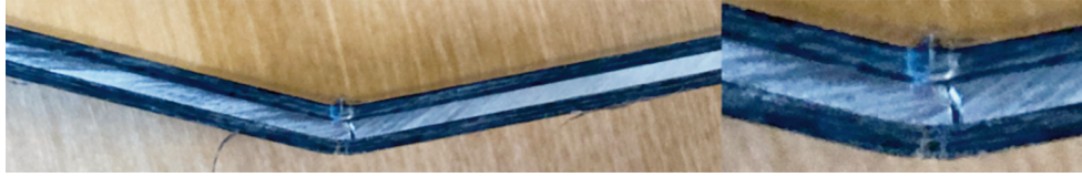
Figure 8. Views of the fatigue damage of the specimen series 2 occurred after 130,000 cycles.
