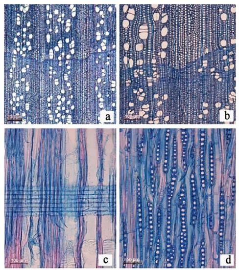
a, b: TS, wood is diffuse porous, the growth ring is obvious, aggregate rays; c: RLS, homocellular rays, vessel, fiber texture, scalariform perforation table in vessel; d: TL, uniseriate-homogeneous rays, type III, fiber texture, and aggregate rays (gathered together).
