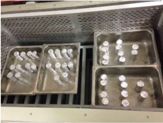
Figure 2: Closed system full automatic freezing–thawing test cabinet.
