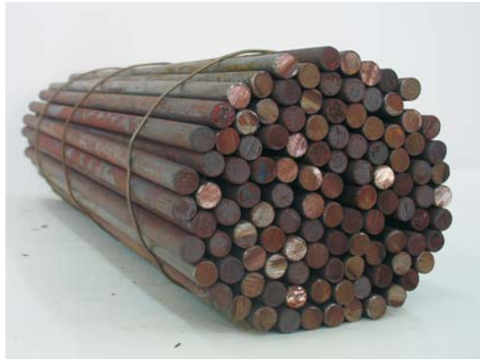
Figure 1. View of a packed bar bundle showing its porous structure.
