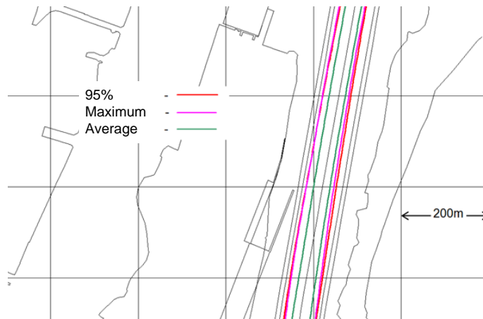
Figure 8. The maneuvering lanes obtained from the container vessel trials with wind speed 5m/s and East direction. Source: Authors.
