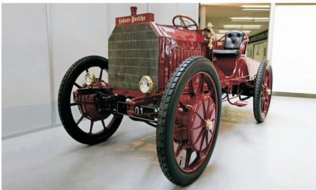
Fig. 1. Lohner Porsche HEV with wheel-hub motor drive [16]
