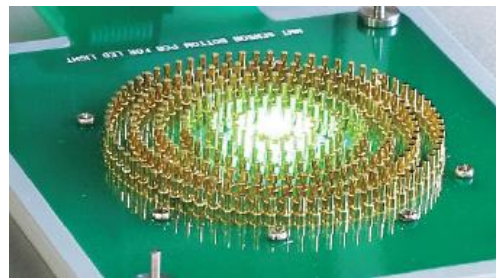
Fig. 3. The bottom sensor of the MMT with the concentric pins.
