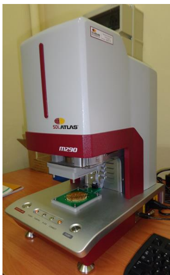
Fig. 1. The Moisture Management Tester M290 by the SDL Atlas Ltd.
