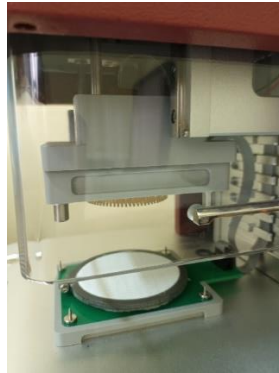
Fig. 6. Stretched sample placed in the measuring area of the MMT.
