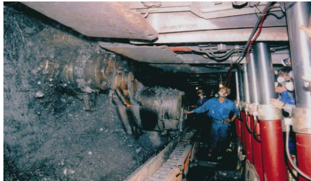
Fig. 5. The mechanized longwall in Khe Cham coal mine [5]
