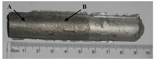
Fig.4. Image of the test alloy ingot with marked areas of microstructure and hardness tests
