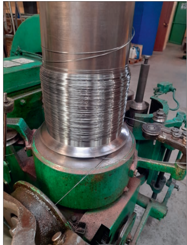
Fig. 6. 25H2N4MA steel wire during drawing with drum-type wire drawing machine
