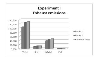
The generated volume of individual harmful products for each of the route is shown in the bar graph (Fig. 6). The defined emission class is Euro 5.
