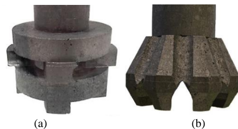
Fig. 3. The impeller variants: (a) F2A 190, (b) J8 190
