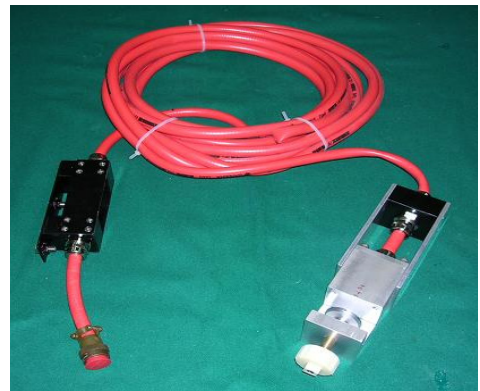
Fig. 3. (photo). Main unit (on the left) and external unit (on the right) of the purpose-built system (Plachno, 2007) for measuring skip's transverse vibration while it traverses the shaft
