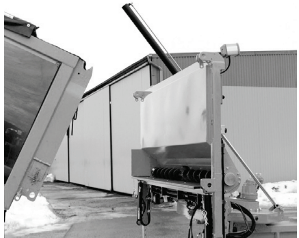
Fig. 7. The set of carrier + hot box + SPRIDER (from the authors' collection).
