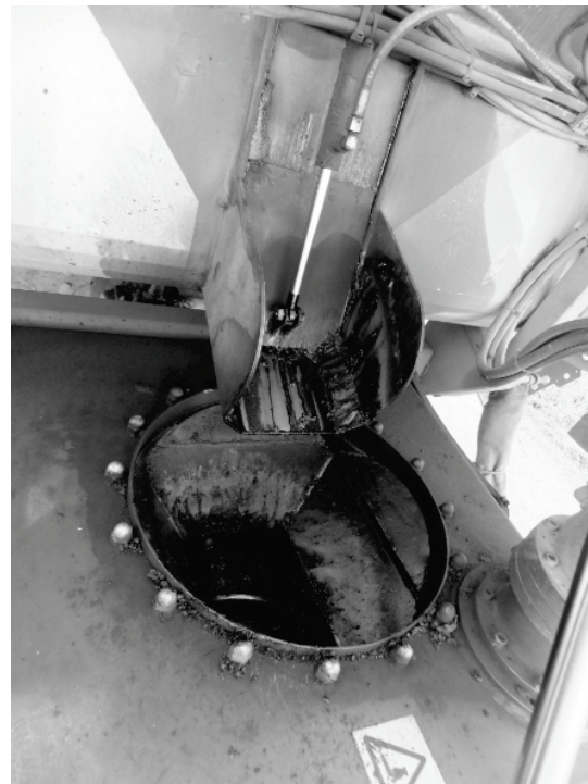
Fig. 10. The arm with conveyor screw, automatic hatch of the SPRIDER (from the authors' collection).
