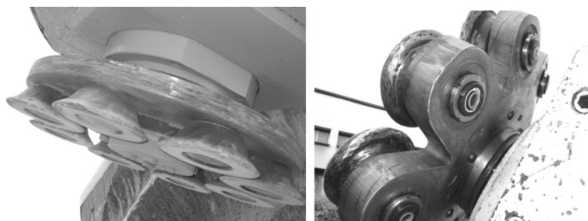
Fig. 5. A view of flat and round plate with traces of wear (left) and new plate in the shape of flower petals (right) (Gospodarczyk et al., 2011)
