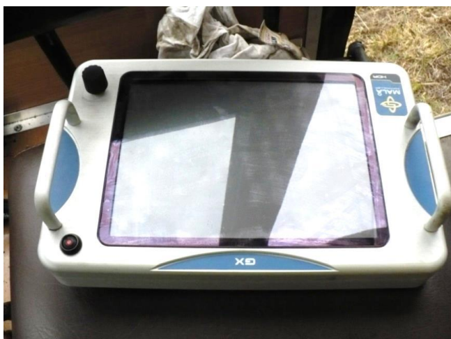
Rys. 3. Georadar Ground Explorer firmy MALA GeoScience.
