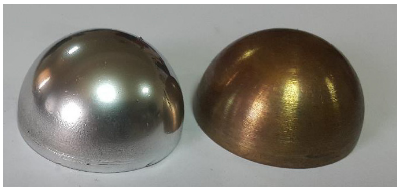
Figure 3. The manufactured zirconium (left) and copper (right) liners
