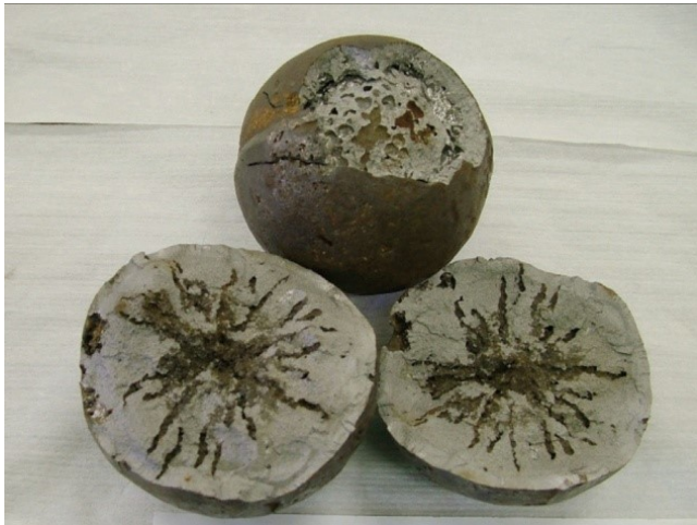
Fig. 4. Shrinkage and gas defects in castings of grinding bodies
