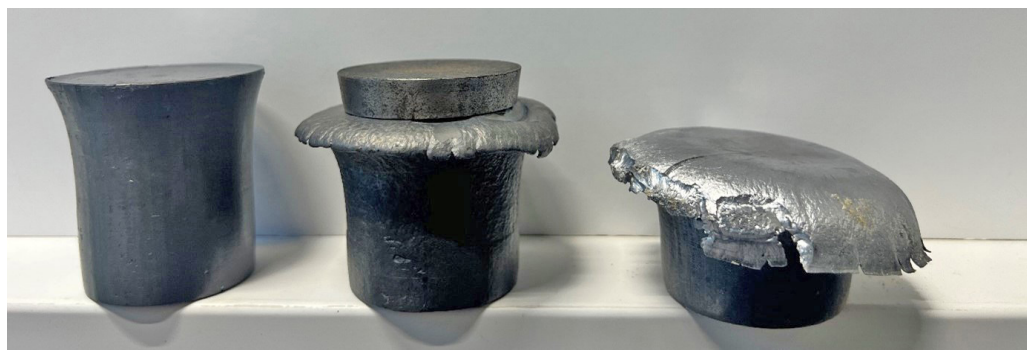
Figure 5. Lead blocks after the tests: ANFO (left), Hydromite 100 (middle) and plastic explosive (right)
