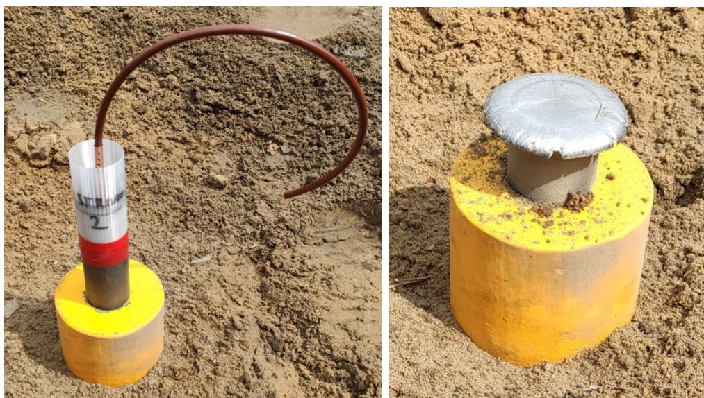
Figure 1. View of the sample prior to firing (left) and lead block after the test (right)
