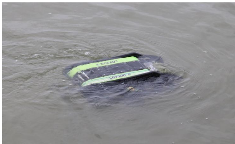
Fig. 5. Remotely operated underwater vehicle with 5 electric propellers propulsion.
