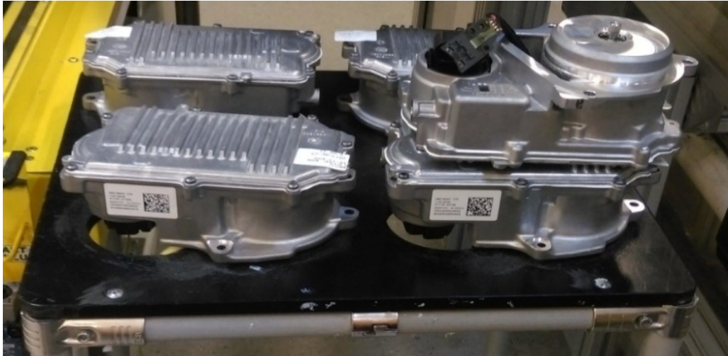
Figure 3. Too small placement area – incorrectly placed part (own study). Source: Doktor, 2018.
