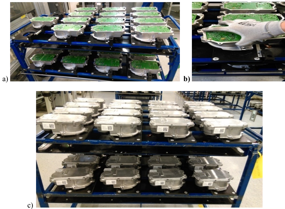
Figure 1. Transport trolleys: a) transport of components, b) collection of components, c) transport of finished products on the soldering line. Source: Doktor, 2018.
