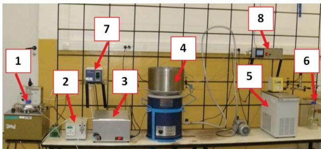
Fig. 1. General view of the test rig: 1. vessel with the tested sample, 2. fuel pump, 3. water bath, 4. sand bath, 5. cooling thermostat, 6. vessel for the tested sample, 7. temperature controller in the sand bath, 8. recorder
