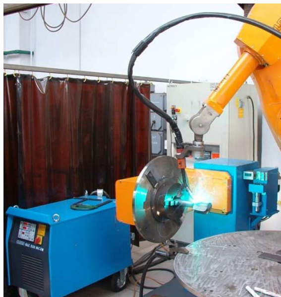
Fig. 2. The robotic welding stand with clamping system
