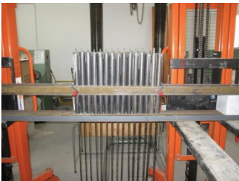
Fig. 1. A stand with unilaterally anchored HFRP bars
