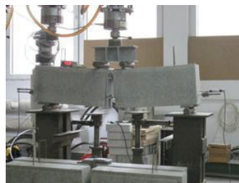
Fig. 4. Loss of bond of an HFRP bar in the final loading stage
