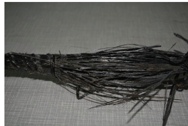
Fig. 2. 14 mm HFRP bars after rupture during a tensile test
