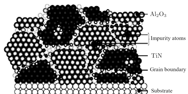
Fig. 2. The model of multiple nano-composite coatings self-microstructure in infancy mutually insoluble phases [12].
